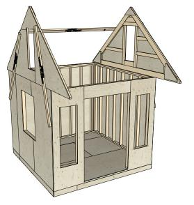
Whether assembling a pre-cut or pre-assembled kit, with or without an enhanced siding package, the walls and gable ends should be erected with the stabalizing effect of either plywood/OSB sheathing or siding already attached. With an enhanced siding upgrade the Ice & Water Shield on the gable ends is attached later in the assembly sequence.
